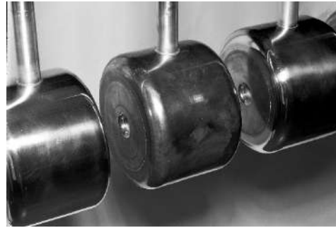
CERN LINAC 4: 352 MHz frequency, Tank diameter 500 mm, 3 resonators (tanks), Length 19 m, 120 Drift Tubes, Energy: 3 MeV to 50 MeV, \beta=0.08 to 0.31 → cell length from 68mm to 264mm.
