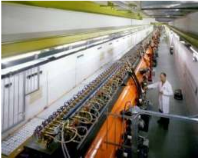
CERN LINAC 2 tank 1: 200 MHz 7 m x 3 tanks, 1 m diameter, final energy 50 MeV.
