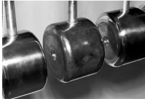
CERN LINAC 4: 352 MHz frequency, Tank diameter 500 mm, 3 resonators (tanks), Length 19 m, 120 Drift Tubes, Energy: 3 MeV to 50 MeV, \beta=0.08 to 0.31 \rightarrow cell length from 68mm to 264mm.
