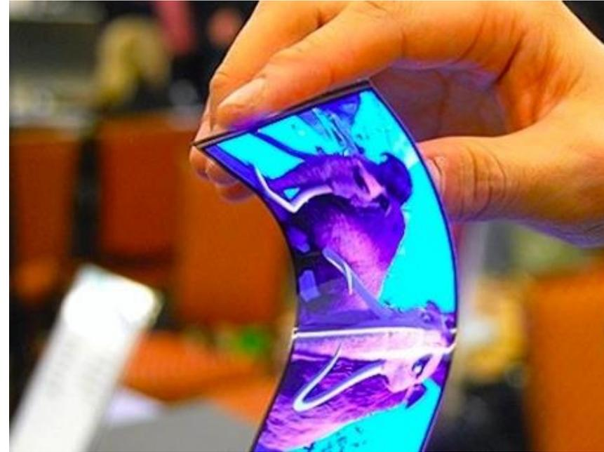
Samsung Flexible Mobile: display technology known as an OLED (organic light emitting diode) (active matrix light emitting diode) screen. As the OLED pixels create their own light source, they don't need a back light like LCD screen technology, but the circuitry to control the pixels is fused into glass.
